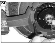
Check the motor for plastic shipping stabilizer tabs, and remove them if they are present. Attach blade assembly to motor by tighten screws securely.
